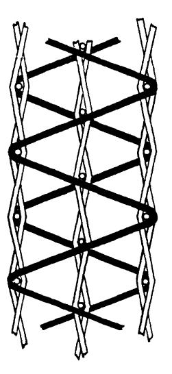
TYPE XX WARP YARNS WEAVING ONE END AS ONE TYPE XXIII WARP YARNS WEAVING TWO ENDS AS ONE BINDER YARNS BOTH TYPES WEAVE ONE END AS ONE
